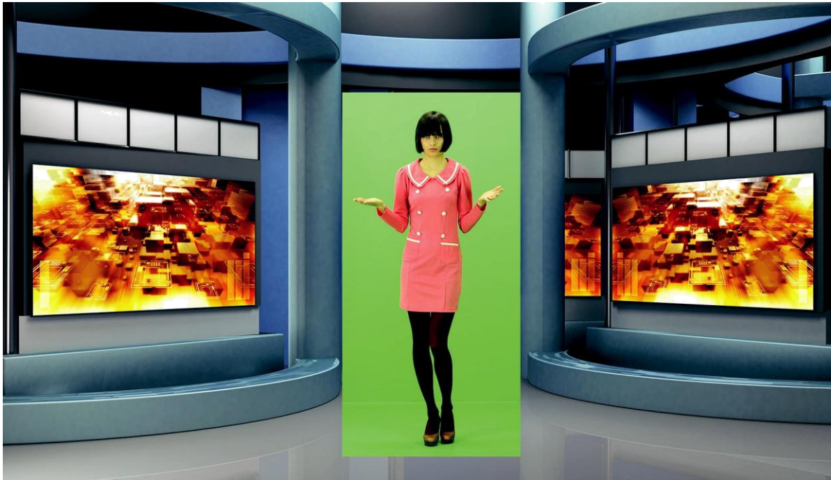
A view after a Garbage mask correction with the keying algorithm switched off
