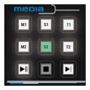
When you select one of the buttons, the illumination of this layer's button changes in the application. Right next to ABCD layer buttons, you can find buttons for setting sources for DSK layers.
