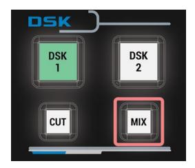
When a proper time is set in the application, the source will appear in a smooth transition from the PREVIEW to the PROGRAM channel.
