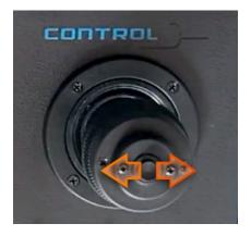
Now let's move the joystick up and down to its extreme positions. When you complete that, the F3 LED will light up in white. Picture below.
