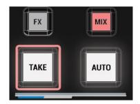
The second method is a transition with the use of AUTO. It is a smooth transition with a time set in the application. After its use, the T-BAR's motion is reflected in the application. And a smooth change between PROGRAM and PREVIEW channels takes place.
