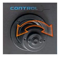
F5 test is the T-BAR's calibration. Move the T-BAR to its extreme positions. Picture below.
