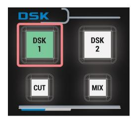
It will be backlit in green, which means - visible in the PREVIEW channel. Now the DELEGATION BUS button is active. Hold down one of the Delegation BUS buttons, e.g. DSK 1. This time you choose a source for DSK 1 in the PREVIEW channel. You can also use the media mixer. Pressing the button brings the
