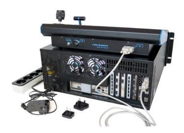
Use a proper power supply adapter used in different types of electrical networks. Select the appropriate adapter and insert it into the power plug. Move it forward until you hear a click. Picture below.
