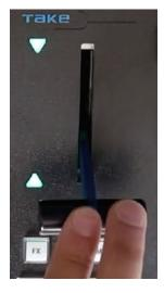
After several movements, all the LEDs will go out. This way, the keyboard has been calibrated and has returned to its normal operation mode.
