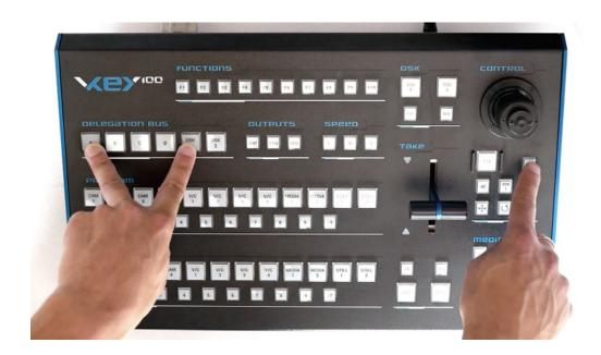
After this pressing, the LOCK and DELEGATION DSK 1 buttons are blinking. It is possible to check the backlight of all buttons. Let's press the keyboard keys one by one, in any order. The first time you press a key, it lights up in white. A second press makes the key light up in its function color. Red, green or orange - depending on its application. Picture below.
