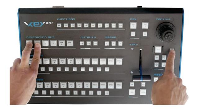
The keyboard shows the current brightness of the keys. Pressing TAKE key several times decreases the backlight's brightness. AUTO key increases brightness of the keys. Picture below
