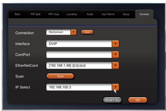
10. Now scroll down the **Connect** tab page to view the switcher's IP information and check if the Model Name displayed is "**SE-500MU**."
