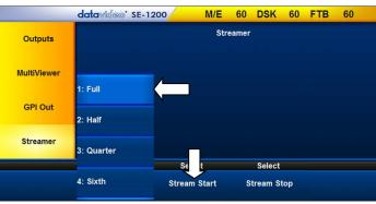
By choosing HALF instead of FULL you are using less bandwidth to support the multi view stream being sent across the IP network.
