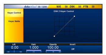
The options in the blue bar along the bottom of the Screen will allow you to calibrate for a white or black key using the **Lift**, **Gain**, **Opacity** and **Invert Functions**. The **Keyer Control section (7.1.1)** will explain the effects of **Lift**, **Gain**, **Opacity** and **Invert**.
