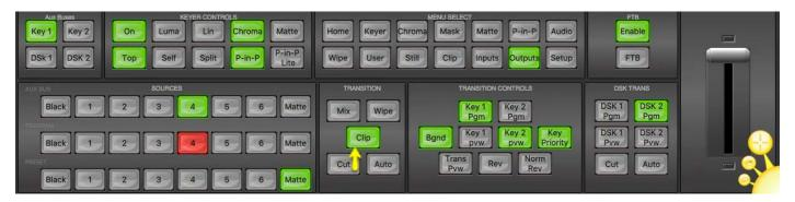
2. Selecting the next source on the lower **Preset row** of buttons and then pressing the **Cut** button.
