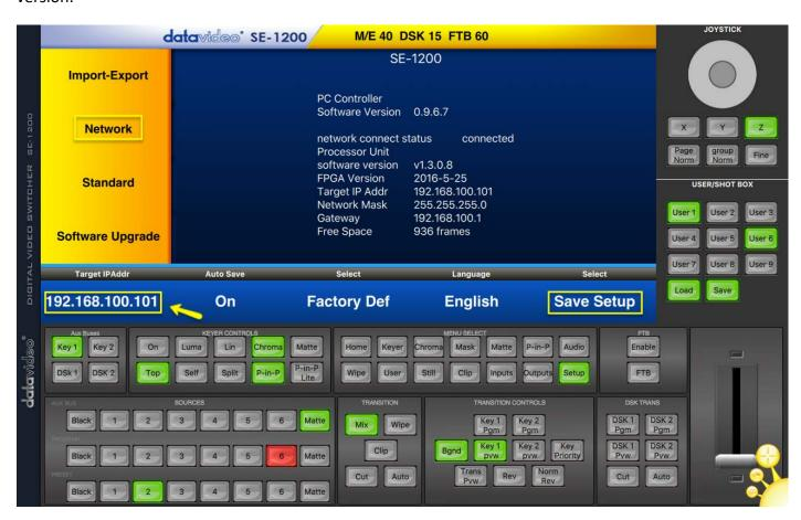
If the network settings are wrong then you may not be able to control the SE-1200 MU. Always keep a note of the last IP settings used and change these settings carefully to avoid problems.
