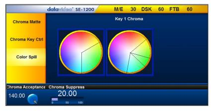
The **Color Spill** parameters and values are shown along the bottom of the display below. These settings are used to control/remove any unwanted Chroma or colour Spill from the background onto the foreground subject. There are two sectors drawn on the **Chroma** palette, one represents the wider **Chroma Acceptance** range and the narrower **Chroma Suppress** range.
