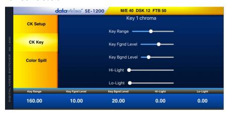
The Chroma Key control parameters and values are shown in the blue bar on the bottom of the screen. Users can control and adjust various parameters such as Key Range, Key Foreground Level, Key Background Level, Hi-Light and Lo-Light by using different sliders shown on the screen respectively.
