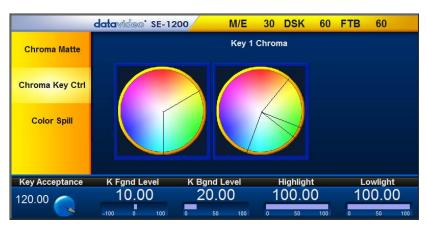
The **Chroma Key Ctrl** parameters and values are shown along the bottom of the display. Two colour palettes, **Main** and **Chroma**, are shown in the diagram.
