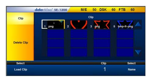
To load the clip, simply click on the **Clip** option and then select "**Load Clip**". The clip is always loaded to input 6 so anything loaded to input 6 before will be replaced by the clip.
