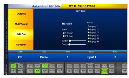
This feature could be used to trigger playback from units such as the Datavideo NVP-20 or HRS-30 or HDR-60/70.
