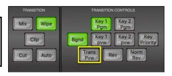
Using the **TRANSITION CONTROLS panel** click to select the **Trans Pvw button** (back lit green is ON). Next select and apply the transition or wipe that you would like to test on the Preview monitor.
