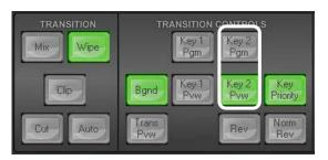
**Step 3:** Turn the Key 2 PIP effect on in the Multi view **Preview output** by clicking the **Key 2 PVW button** (backlit green) in the **Transition Controls panel**.
