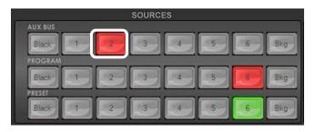
**Step 4:** Select the PiP image source on the **AUX BUS row** of the **SOURCES** panel. This will be shown over the chosen Preview image before being taken to Program/air with the next mix or wipe transition.
