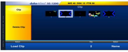
To load the clip, simply click on the **Clip** option and then select "**Load Clip**". The clip is always loaded to input 6 so anything loaded to input 6 before will be replaced by the clip.
