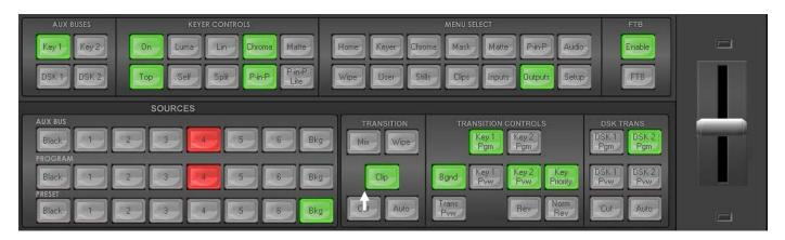
2. Selecting the next source on the lower **Preset row** of buttons and then pressing the **Cut** button.
