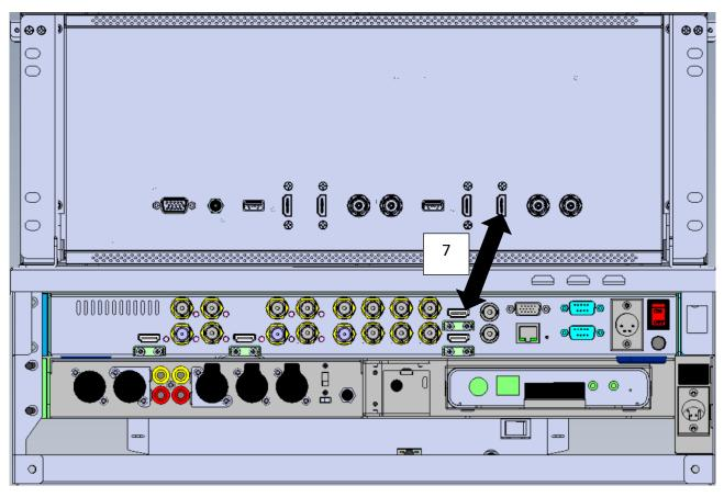
3. Please connect the Cable No. 8 (HDMI Cable) from the PGM HDMI OUT interface on the rear panel of the KMU-100 to the HDMI IN interface on the rear panel of the NVS-30.
