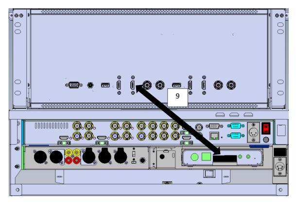
5. Please connect the Cable No. 10 (RCA Cable) from the RCA output interface on the rear panel of the AD-100M to the 3.5mm unbalanced analog audio input interface on the rear panel of the NVS-30.
