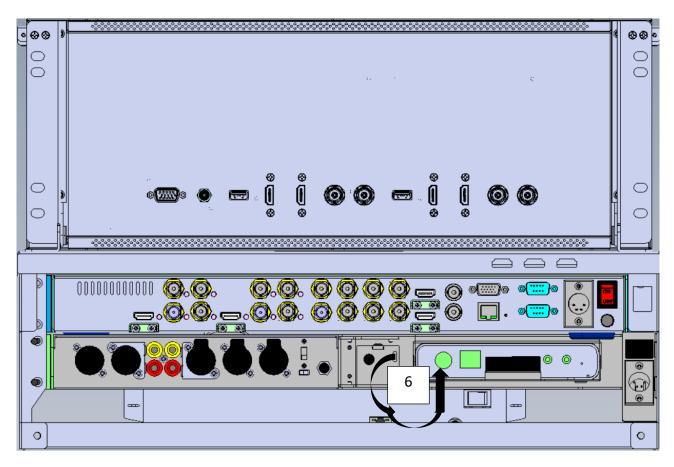
2. Please connect the Cable No.7 (HDMI Cable) from the Multiview HDMI OUT interface on the rear panel of the KMU-100 to the HDMI IN1 interface on the rear panel of the TLM-102.
