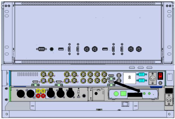
4. Please connect the Cable No. 9 (HDMI Cable) from the HDMI OUT interface on the rear panel of the NVS-30 to the HDMI IN2 interface on the rear panel of the TLM-102.
