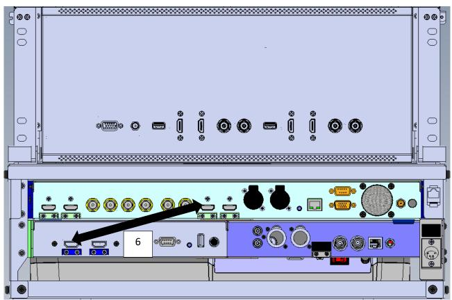
2. Please connect the Cable No.7 (HDMI Cable) from the HDMI OUT interface on the rear panel of the HDR-1 to the HDMI IN2 interface on the rear panel of the TLM-102.
