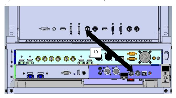
6. Please connect the Cable No. 11 (Ethernet Cable) from the LAN interface on the rear panel of the NVS-25 to the RMK-6's RJ-45 interface on the inner side of the RMK-6.
