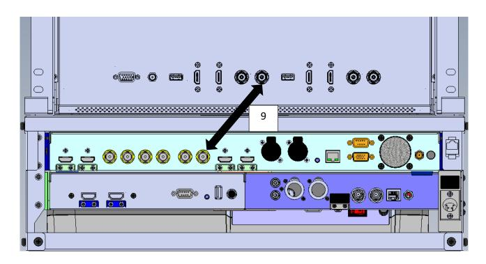
5. Please connect the Cable No. 10 (BNC 180 Degree Cable) from the SDI OUT 2 interface on the rear panel of the TLM-102 to the SDI IN interface on the rear panel of the NVS-25.
