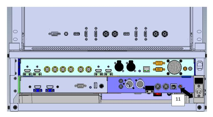
7. Please connect Cable No. 12 (D-sub 9 pin male to male cable) from the RS-232 interface on the rear panel of the RMC-260 to the RS-232 interface on the rear panel of the SE-1200 MU.
