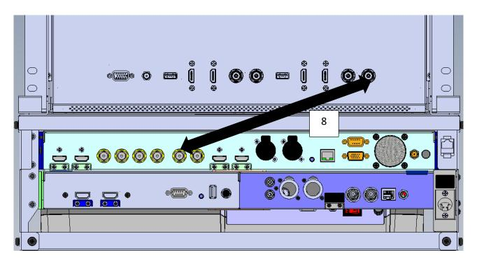
4. Please connect the Cable No. 9 (BNC 180 Degree Cable) from the SDI OUT2 interface on the rear panel of the SE-1200 MU to the SDI IN2 interface on the rear panel of the TLM-102.
