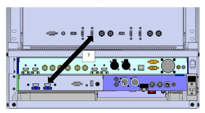
3. Please connect the Cable No. 8 (BNC 180 Degree Cable) from the SDI OUT1 interface on the rear panel of the SE-1200 MU to the SDI IN1 interface on the rear panel of the TLM-102.
