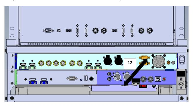
8. First locate the DC jack on the RMK-6 and on the inner side of the DC jack, you should find five DC plug cables attached. Connect Cable No. 1/2/3/4/5 (DC Plug Cable) to the RMC-260, TLM-102, NVS-25, HDR-1 and SE-1200 MU DC jacks respectively and secure by tightening the outer fastening ring.
