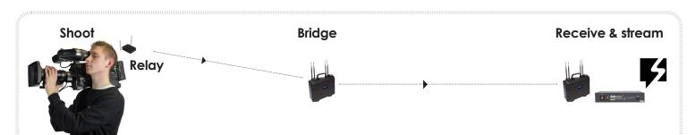
Send an H.264 signal from an HD camcorder to the production desk at distances of over 250m using IntraTec Bridge and a mini encoder. The wireless signal is received by the battery operated NVW-250 which houses a mini decoder, Duo also supplies a power source for a Datavideo handcarried switcher and the decoder.
